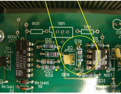
To modify the gain, replace resistor R10 with a  $150k\Omega$  resistor
